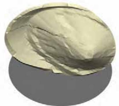
Above: Profile scan of a 30m diameter bin at various stages during storage.
